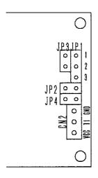
The following table shows the function of No1 and No2 of JP1, JP2. CU16025ECPB·W6J is no reset inputs from third hole of 14 through holes and M68 CPU bus interface. Reset input signal is active when it is low.
